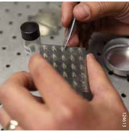
The SwRI method allows batch testing. Microspheres loaded into this miniature series of “barrel” holes allow the system to automatically fire them in rapid succession.
