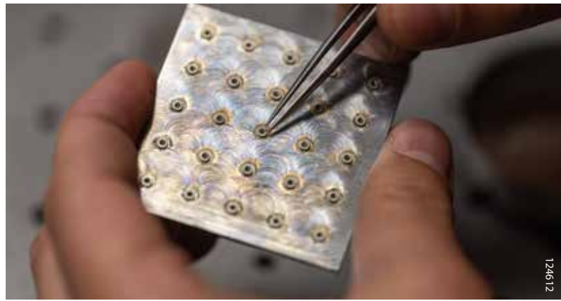
The SwRI method allows batch testing. Microspheres loaded into this miniature series of “barrel” holes allow the system to automatically fire them in rapid succession.
