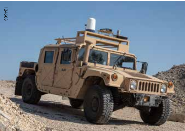
SwRI developed a Vision for Off-Road Autonomy (VORA) tool, a passive camera system to perceive objects, model environments and simultaneously localize and map while navigating off-road environments — including exploring planetary surfaces, as demonstrated here at an analogous Earth setting.
